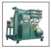
**Brief introduction:** This series of machines are originated products in China developed t meet the needs of insulation breakdown test under various conditions (especially in field operations). The can test the filtration effect and may completely take the place of traditional breakdown testing equipment.
