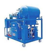
**Brief induction:** Higher than the national standard, the machine can raise breakdown voltage by 35KV at one time and reduce aging harm due to repeated filtration and heating with a common oil filter.
